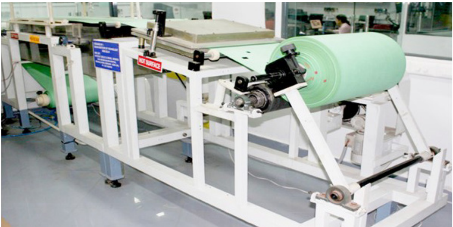
Figure 1: Continuous Electrospinning Machine (Lab Prototype) Developed by IIT Delhi Researchers
