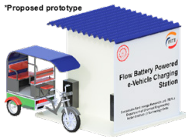
Figure 4. VRFB based Charging Station (under development)
