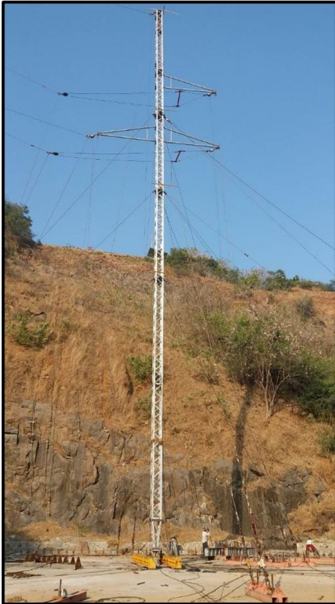
Fig. 5a. Prototype test of ERS for 220 kV single-circuit TL tower
